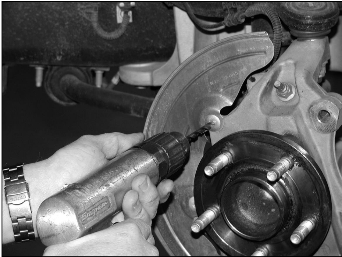
Figure 1: Drilling out each rivet
