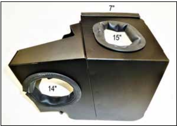
9. Install the shorter edge trim into the heat shield as shown.
