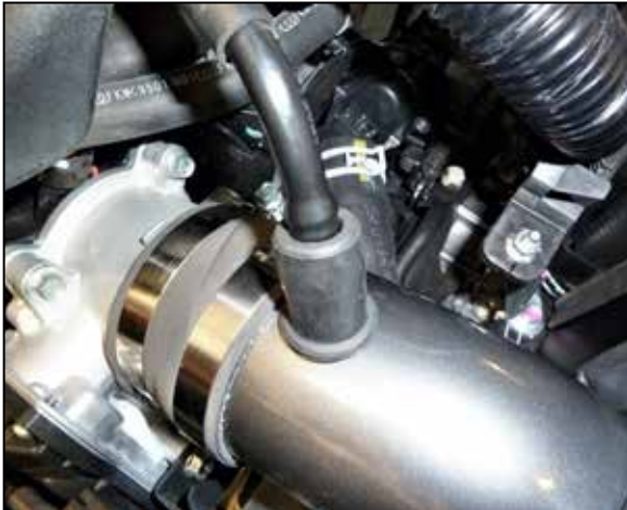
15. Install the factory ccv pipe into the grommet installed into the K&N intake tube.
