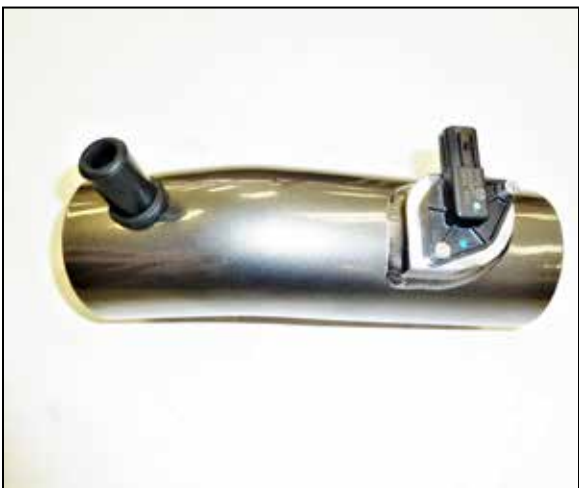
13. Remove the maf sensor from the factory air filter housing and then install it into the K&N intake tube. Install the provided ccv grommet into the intake tube and then install the provided TYPHOON decal.
