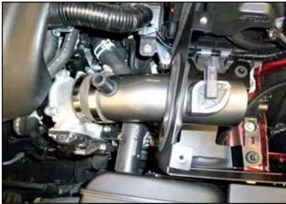
14. Install the K&N intake tube assembly through the heat shield and into the coupler at the throttle body, adjust the tube for best fit and then secure with the provided hose clamp.
