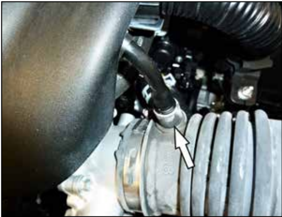
5. Loosen the hose clamp that secures the intake hose to the throttle body and then disconnect the CCV pipe from the intake hose. Lift the complete intake assembly up and remove it from the vehicle.
