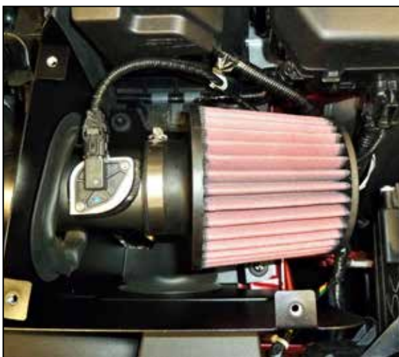
16. Install the AEM air filter onto the intake tube and secure with the provided hose clamp. Reconnect the maf sensor electrical connection.
