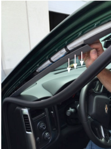
1. Pull door weather strip down and away from trim.
