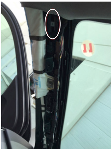
4. Insert the supplied well nut into the slot as shown.
