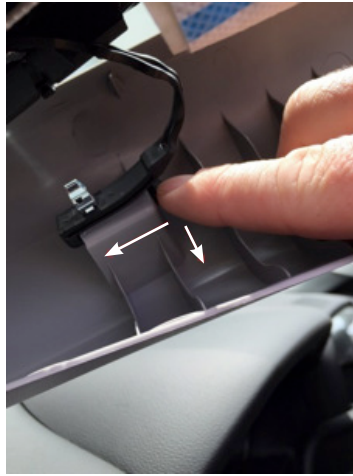
2. Release clip by pressing down, then forward.
