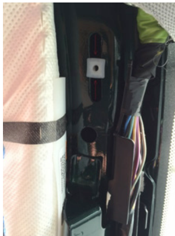
5. Be sure to fully seat and center the nut.
