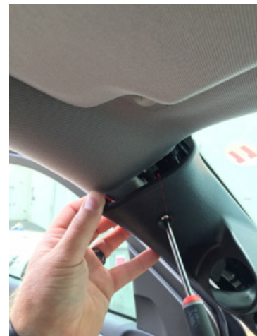
6. Install the bottom portion of the pillar. Thread screw into well nut about 2 turns.
