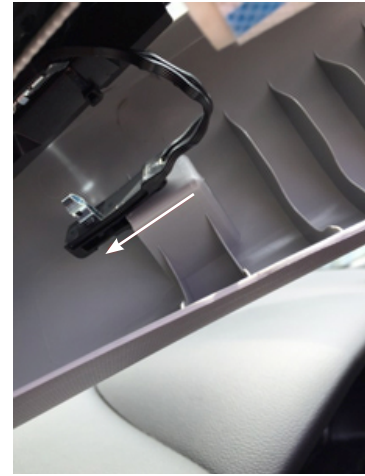
3. Clip will slide off of pillar, allowing pillar to be removed.
