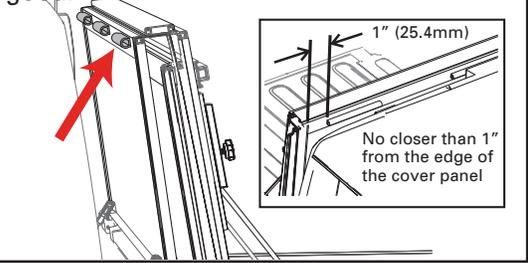
**11** Unfold the cover (A) towards the tailgate. Then confirm each panel is centered side to side and front to back on the truck bed. If adjustments are needed, loosen the cover retainer clamps (E) and shift the cover until positioned correctly. The rear edge of the cover and tailgate seal should rest on top of the tailgate. For proper sealing, the tail panel will overlap by .5".
