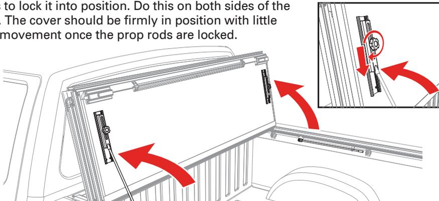
Before flipping cover (A) in the up position make sure to stow the straps using the clips on the underside of the folded cover.
