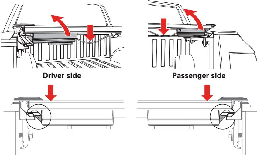
**13** Retighten the cover retainer clamps once the desired fitment is reached. **You are ready to drive with your cover in the closed position.**
