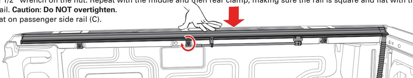
**NOTE:** If the rails are leaning down, have one person stand on the outside of the bed and slightly roll the rails upward while another person slowly snugs the clamps up. If the clamps are tightened too quickly or overtightened, it will cause the rails to lean down.
