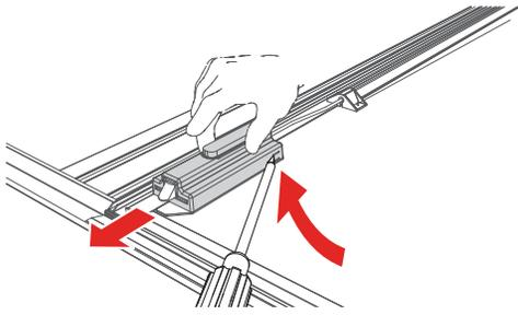
Use a screwdriver to partially pry open the tab on the latch housing. At the same time slide the housing away from the latch assembly.
