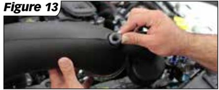
**6.** Install the Banks intake tube. First insert the tube into the air filter opening. Next insert the tube into the Banks hose at the throttle body. See **Figure 14**
