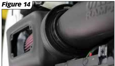
**NOTE:** Take care not to pinch or trap the pcv line under the tube. Line up the arrows on the filter and tube before tightening all 3 hose clamps.
