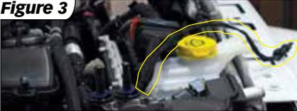
**3.** Unhook the coolant hose from the factory intake tube if equipped.
