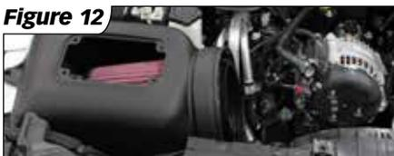
**5.** Install the supplied grommet into the IAT port in the Banks intake tube. See **Figure 13**
