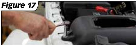
**10.** Install the Banks window onto the housing using a phillips screwdriver and the 4 supplied screws. Apply the supplied thread locker on the screws to prevent them from backing out over time.
