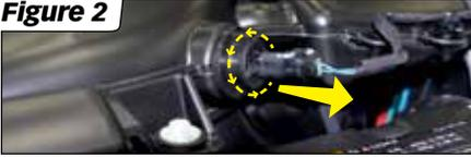
**2.** Unhook the 2 clips securing the IAT harness to the factory intake tube. Pull the sensor and harness out of the way. See **Figure 3**
