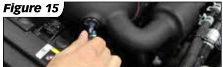
**8.** Push the PCV line onto the aluminum fitting of the Banks intake tube. See **Figure 16**
