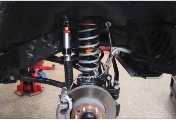
13. Release the spring compressors allowing the spring to sit in the upper isolator and lower perch.
