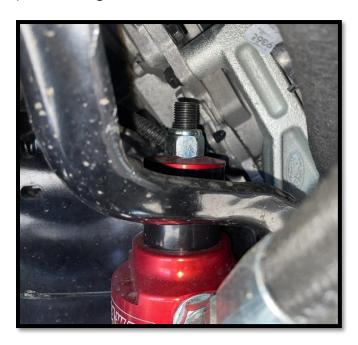
17. Using the included hose clamps and an **8mm** socket, mount the shock reservoir to the reservoir bracket as shown in the below photos.
