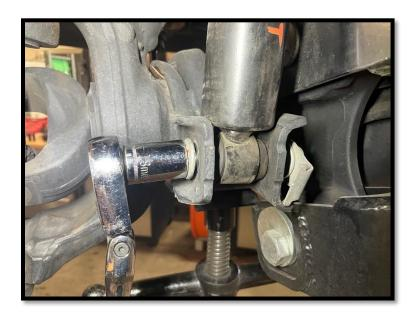
9. Using a **19mm** wrench, remove the upper shock nut and bushing, then lower the shock rearwards to fully remove it from the vehicle.
