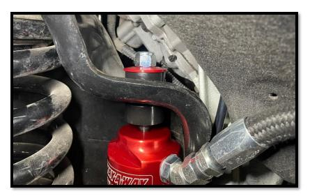
15. Using an **18mm** socket, install the lower shock bolt through the lower eyelet and misalignment spacers of the shock. You may need to raise or lower the axle slightly to align the bolt with the eyelet. Torque the lower shock bolt to 111 ft\*lb (Reference the factory specification shown in the table on the last page).
