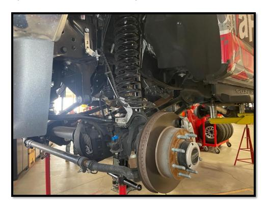
3. Using an **18mm** socket and **8mm** wrench, remove the sway bar end link upper nuts.
