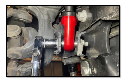
16. Using a **19mm** wrench and **1/4**" Allen wrench, tighten the upper shock nut, compressing the bushings approximately 3/16", until the red washer engages with the inner bushing sleeve. The nut will not tighten past this point.
