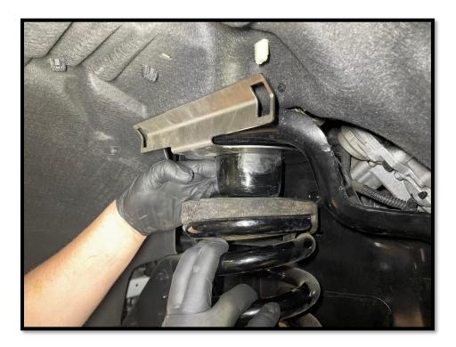
12. Verify that the lower spring pigtail is properly indexed with its axle seat as shown in the below photo.
