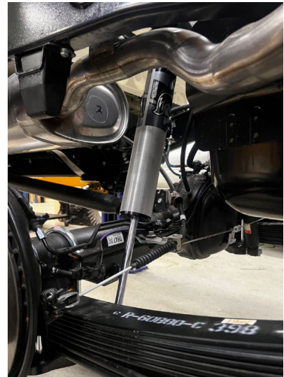
Fig. 3: Rear Fox shock installed
