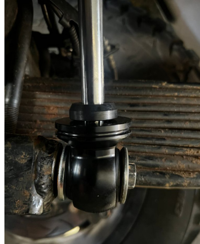
Fig. 2: Rear Fox shock, lower eyelet
