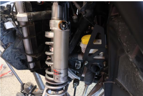
Set the adjuster to 7 clicks clockwise from the full open (soft) position.
