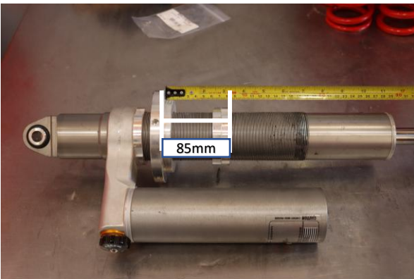
Set the crossover ring to 85mm (3 11/32") front the spring seat to the bottom of the crossover ring.
