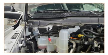
**11.** Remove the three (3) nuts securing the stock tank to the vehicle and remove the tank.
