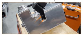
**13.** Install the Mishimoto tank onto the vehicle and secure it with the three (3) nuts removed in Step 11.
