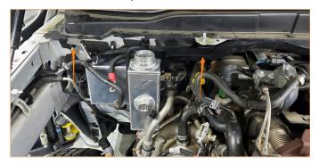
**14.** Connect the stock level sensor plug to the plug on the level sensor installed in the Mishimoto tank.
