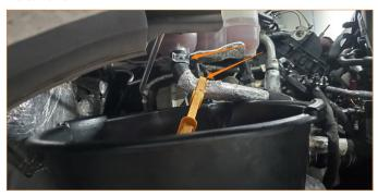
9. Remove the tree clips securing the upper tank hoses from the tank.
