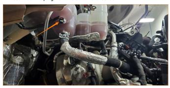
8. If not draining the entire cooling system, pinch off the lower expansion tank hose. Place a container under the expansion tank and remove the hose clamp and hose from the tank to drain it into the container.
