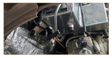
15. Connect the lower tank hose to the Mishimoto expansion tank.
