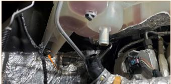
**12.** Using the two (2) supplied M6 bolts, flat washers, & lock washers, attach the mounting bracket to the Mishimoto expansion tank.
