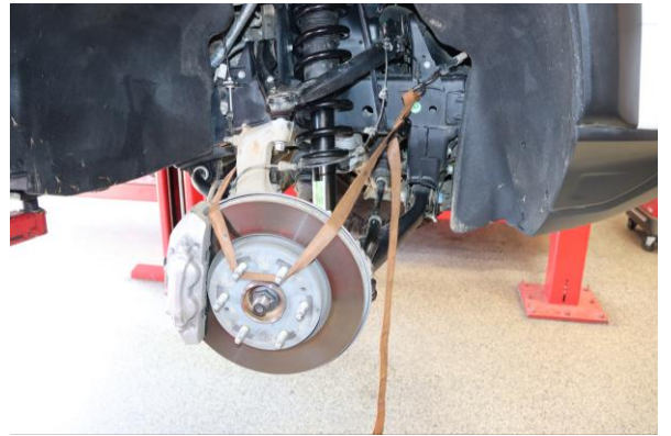
Step 4. Use a strap to prevent over extension of the axle during shock removal and installation.
