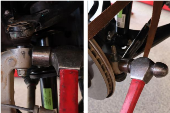
Step 7. Use a hammer to shock and separate the upper ball joint and outer tie-rod end.
