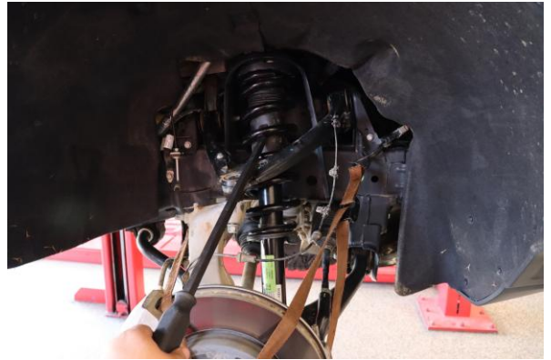
Step 8. Use a pry bar to lower the upper control arm. Remove the 18mm upper ball joint nut. Slowly allow the upper control arm to lift out of the steering knuckle. Allow the knuckle to rest against the strap installed in step 4.
