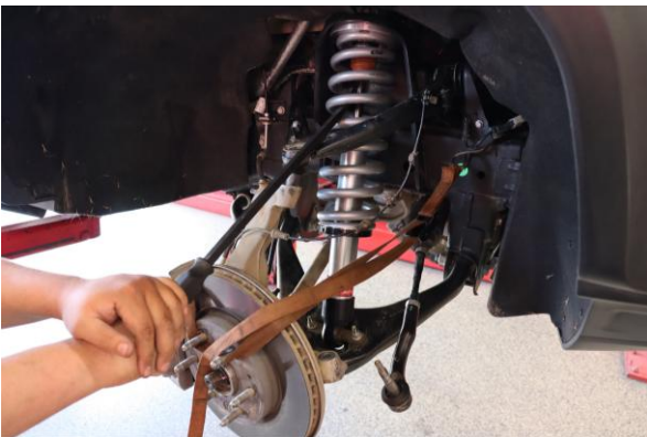
Step 17. Use a pry bar to lower the upper control arm and ball joint into the steering knuckle. Install and tighten the 18mm ball joint nut to manufacturer specification.
