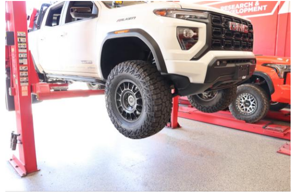
Step 20. Install wheel and tire. Tighten 21mm lug nuts to manufacturer specification.
