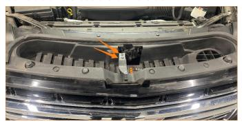
**3.** Remove all 9x push clips that secure the upper radiator panel to the vehicle and remove the panel from the vehicle.
