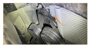
**10.** Inspect the seal on the transmission lines and make sure that it is present and clean. Reinstall the transmission lines and secure them with the included bolts. Tighten the 13mm bolts to 16 ft-lbs. (See next page)
