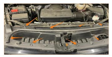
4. Remove the 2x 13mm bolts that secure the radiator support tie bars to the radiator support and move them down and out of the way. Unclip the hood latch release cable from the clip to move it out of the way.
