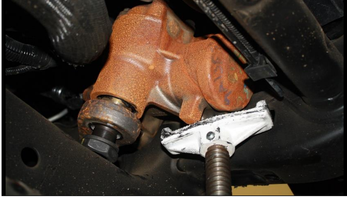
Figure 4: Support the Steering Box with a Jack
