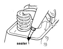
PRIOR TO INSTALLING VALVE COVER apply a small dab of silicone sealer where all gaskets and seal(s) meet.
