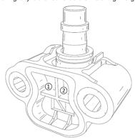
Install the gasket by pressing in the two rubber blocks into the upper left and right cross-member of the tensioner body (1) & (2)).
