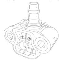
Install the gasket by pressing in the two rubber blocks into the upper left and right cross-member of the tensioner body ( $\bigcirc$ ).
