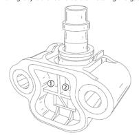
Install the gasket by pressing in the two rubber blocks into the upper left and right cross-member of the tensioner body (1) & (2).
