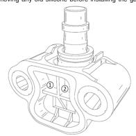
Install the gasket by pressing in the two rubber blocks into the upper left and right cross-member of the tensioner body ((1) & (2)).
