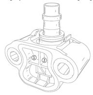
Install the gasket by pressing in the two rubber blocks into the upper left and right cross-member of the tensioner body ( $\bigcirc$ ).
