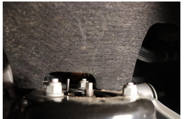
12. Remove the upper shock mount nuts with a 15mm wrench.
