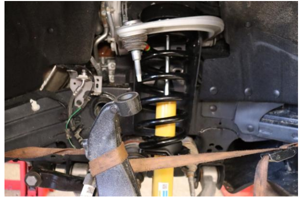
8. Remove the upper control arm from the steering knuckle
