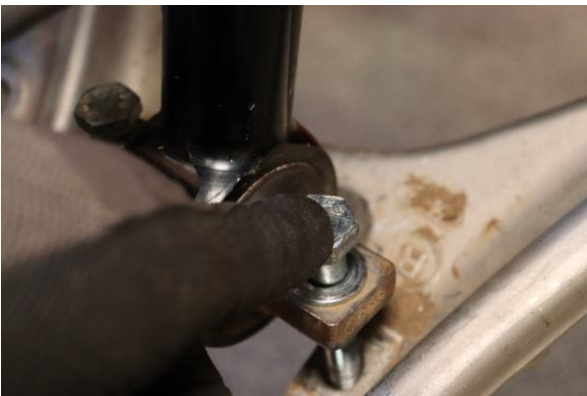
17. Install the lower shock mount with the provided hardware kit.
