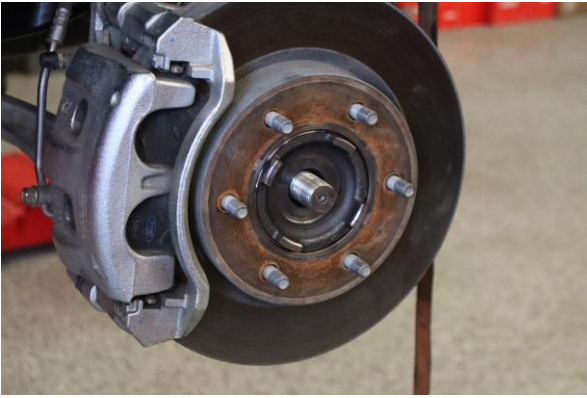
19. Reinstall the axle shaft into the hub.
