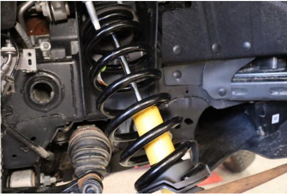
13. Remove the front shock assembly.
