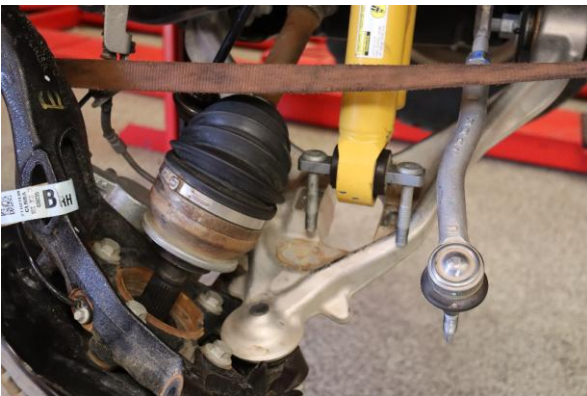
11. Lower the lower control arm and fully remove the axle and lower shock mount.
