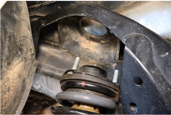
8. Remove the rear shock assembly.
