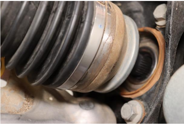
9. Remove the axle from the knuckle.
