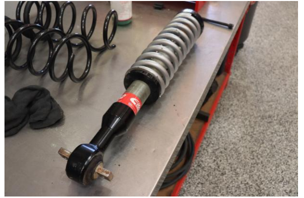
14. Set the front coilover assembly to the desired height before installation. Ensure that both coils are set to the same height. Out of the box heights and adjustment recommendations can be found in the table at the end.
