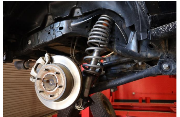
9. Install the rear coilover.
