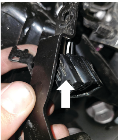
Fig. 10c: Lift the tab to remove the connector
