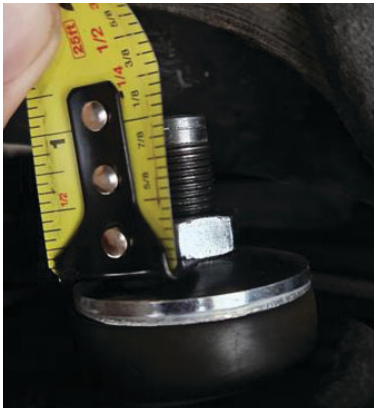
Fig. 36a: Install the jam nut
