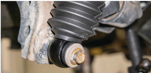
Fig. 35: Install the lower shock bolt
