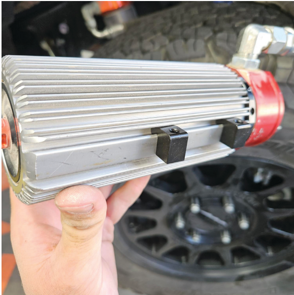
Fig. 37: Assemble the hooked clamps to the top rail of the reservoir's doetail
