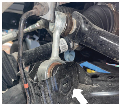
Fig. 2b: Sway bar end link (non-KDSS)
