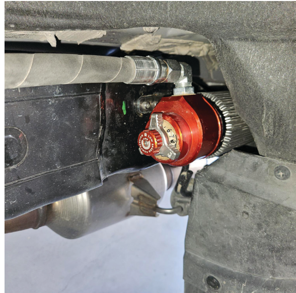
Fig. 38: Assemble the reservoir onto the bracket.
