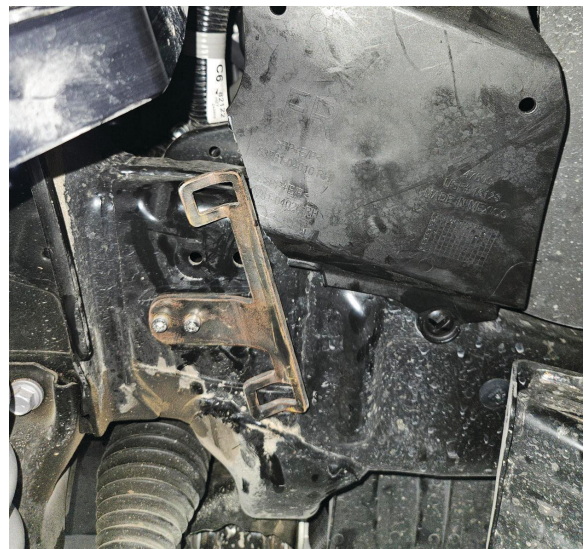
Fig. 20b: Cut the splash guard
