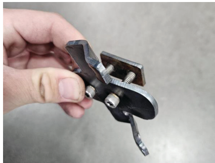
Fig. 6: Pre-assemble the bracket assembly
