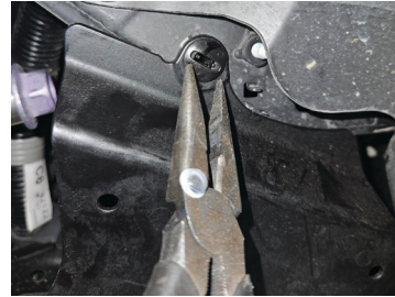
Fig. 5: Remove the splash guard
