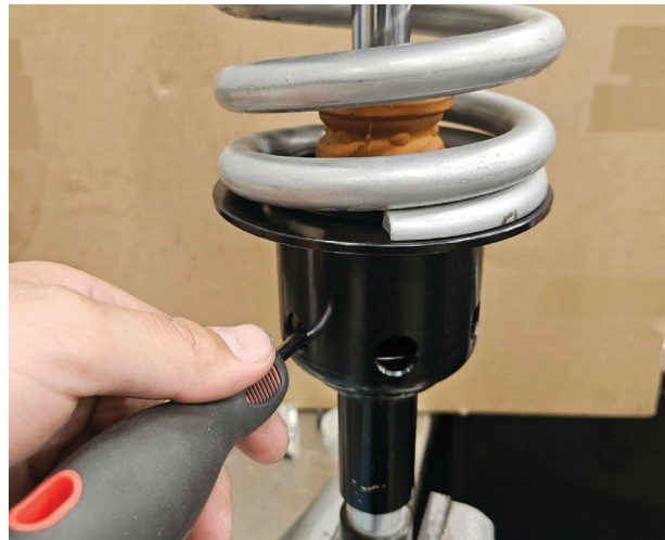
Fig. 24: Lift the bump stop with a screwdriver.
