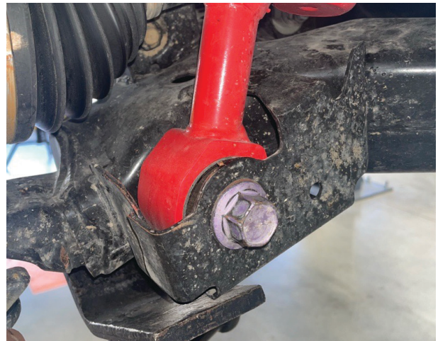
Fig. 14: Remove the bolt from the lower control arm.
