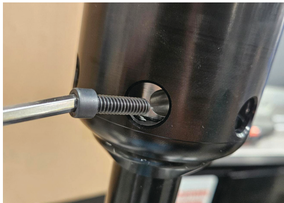
Fig. 26: Screws to clamp spacers to shaft.
