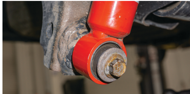
Fig. 29: Remove lower shock mount bolt.
