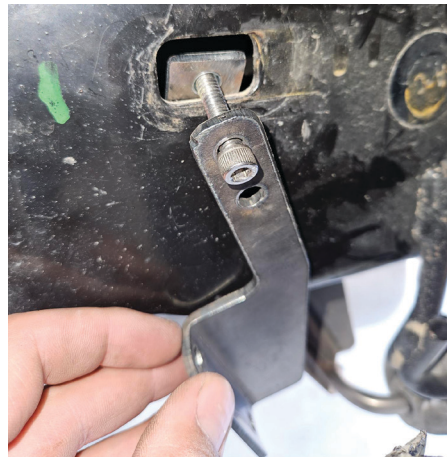
Fig. 32: Insert the nut plate
