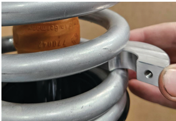
Fig. 25: Slide spacers through spring.
