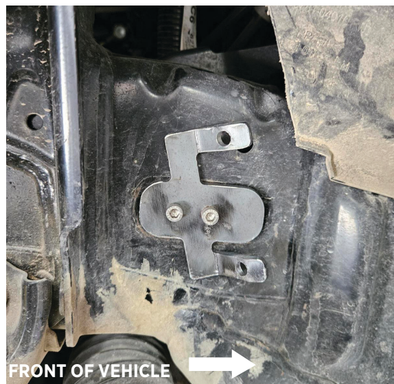
Fig. 7: Adjust the bracket and tighten the screws
