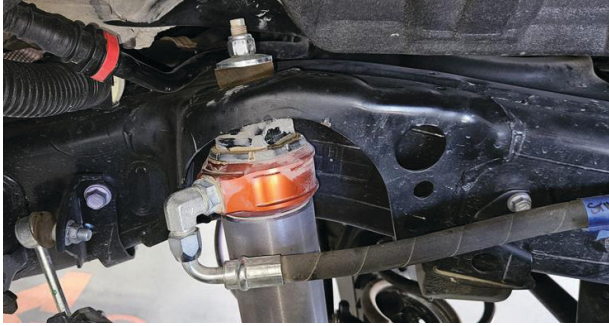
Fig. 34: Install the stem top nut (driver side shown).
