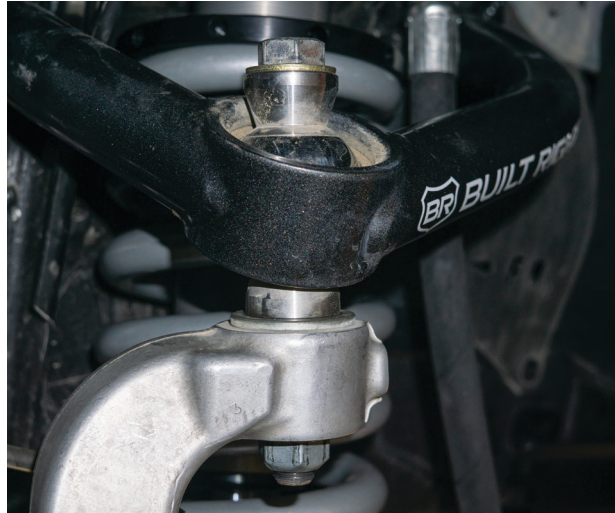
Fig. 21: Reattach UCA to the upright.
