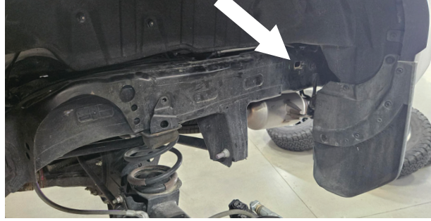
Fig. 30: Remove the rear plastic plug
