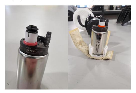
6 – Install the pump into the center section, all 3 of the O-rings should be seated inside the inlet of the module center section, lock the pump into place by latching the three lock tabs on the filter sock retainer.
