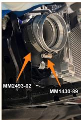
30. Install the Mishimoto cold side pipe into the vehicle.
