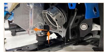
19. Loosen the clamp on the cold side charge pipe, and then remove the pipe from the vehicle.
