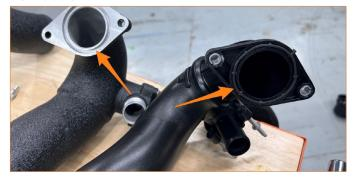
28. Install the upper section of the Mishimoto charge pipe in the vehicle by feeding the bead rolled end under the harness and rotating it into position onto the mounting studs.
