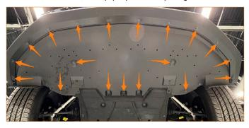
2. Remove the 6 pop clips from the left side wheel liner. Repeat this for the right side, and then remove the splash guard from the vehicle.
