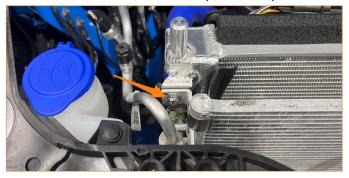
16. Release the clips on the 2 quick-disconnect fittings and pull them off the intercooler. Unplug the electrical connector for the pressure sensor.
