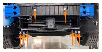
11. Unplug the electrical connector "A", remove the 3 harness tree clips "B", and remove the 2 bolts "C" (8mm socket). Remove the grill shutter assembly and the lower brace from the vehicle.
