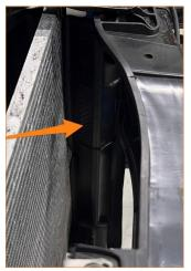
14. Remove the 4 bolts for the 2 radiator brackets, and then remove the brackets.
