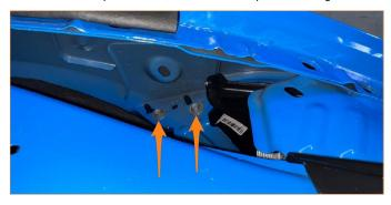
6. Remove the 6 bolts from the upper part of the bumper (10mm socket) then remove the bumper.
