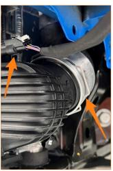
33. Install coupler 2 between the throttle body and cold side charge pipe. Fasten the coupler with an 89mm worm gear clamp and a 76mm worm gear clamp.
