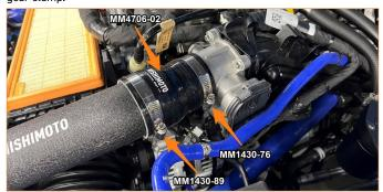
34. Fasten the upper section of the hot side charge pipe using the 2 stock nuts. Tighten the 2 89mm worm gear clamps on coupler 1.
