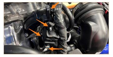
24. Loosen the 2 clamps and remove the hose. Note: clamps are different than pictured.
