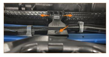
8. Remove the 3 tree clips fastening the ducting around the grill shutter assembly.
