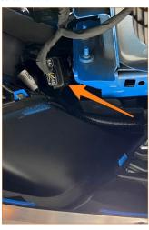
4. Remove the 8 pop clips from the plastic radiator cover then remove the cover from the vehicle.
