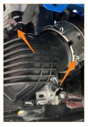
17. Release the intercooler from the radiator by pulling down on the lock tabs and then pulling forward on the bottom of the intercooler. Remove the intercooler by lifting the whole assembly up over the hooks on the radiator then removing it out the front. Note: you may have to lift up on the AC condenser.
