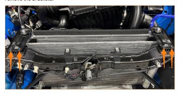
15. Remove the bolt from the AC condenser (10mm wrench).
