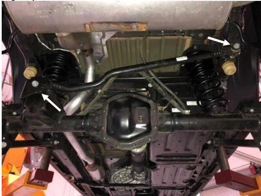
Track Bar Bolts
