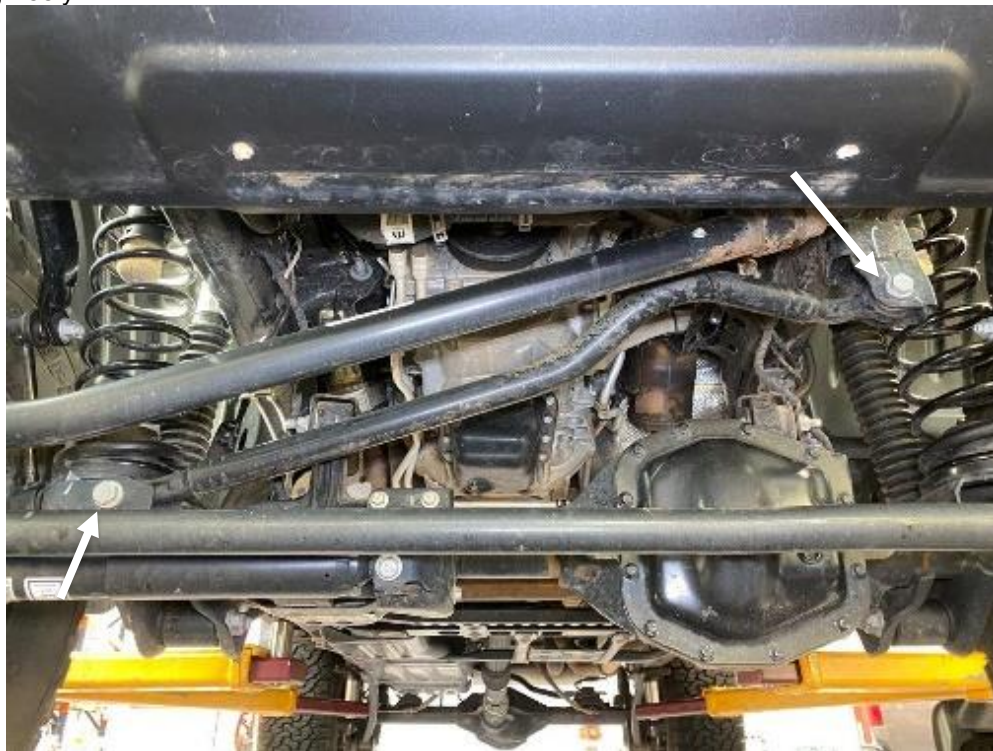
Track Bar Bolts
