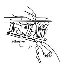
**ATTACH AND ALIGN GASKET(S):** Apply quick drying adhesive sparingly in several places on the engine casting or oil pan (depending upon engine model). Mount gasket on surface where adhesive was applied.
