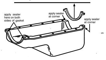
**PRIOR TO INSTALLING OIL PAN GASKET** apply a small dab of silicone sealer to the 4 corners of the oil pan.
