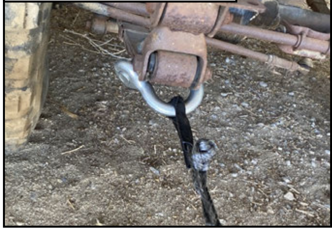
Figure 21b –Utilize a steel shackle when securing the winch line to sharp edges
