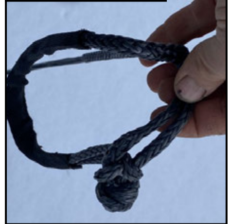
Figure 22c –Pull the soft shackle tight to secure
