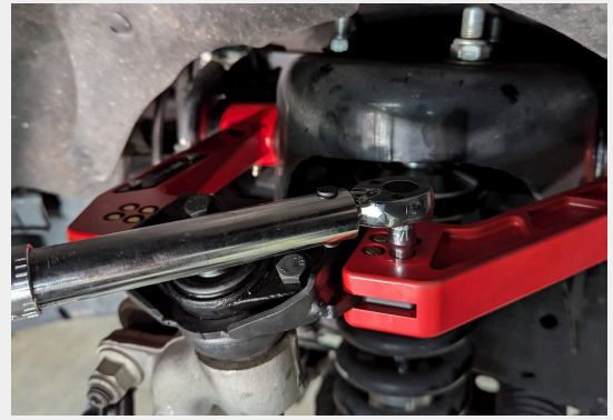
Figure 6: Double check Ball joint pad Torque.
