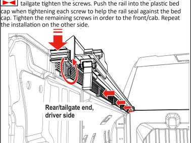
Install the remaining four middle clamps. Starting with rear/
