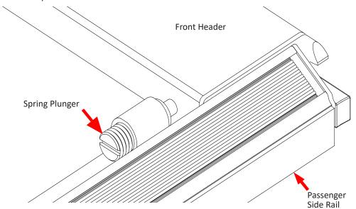
**NOTE:** Check cover tension after installation, seasonally, and after extreme temperature changes.
