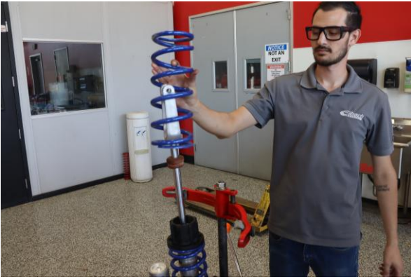
Remove the OE main spring.
