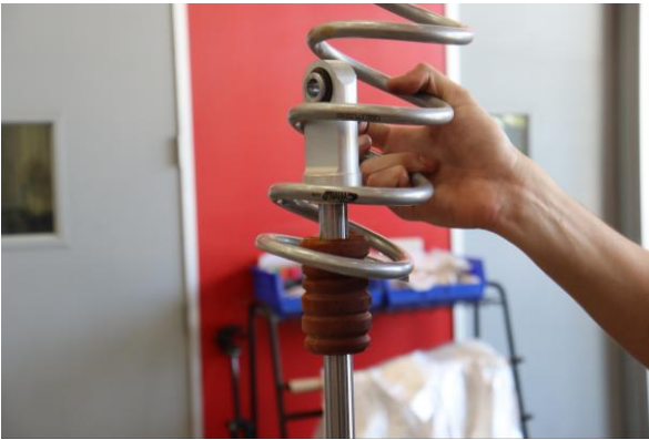
Install the Eibach rear tender spring.
