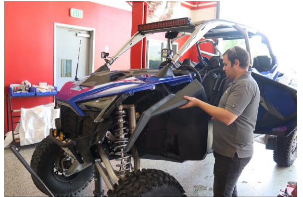
Remove the fender.
