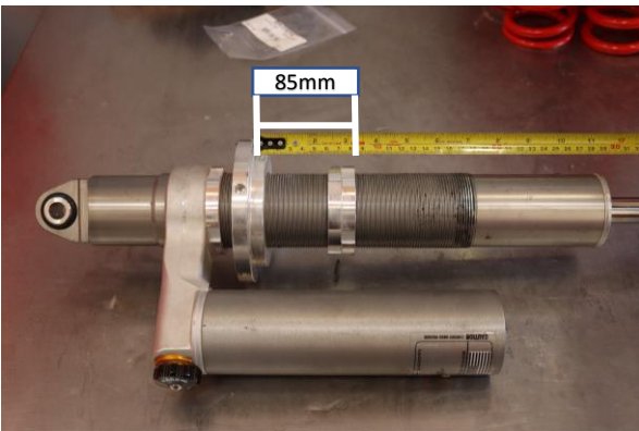
Set the crossover ring to 85mm (3 11/32") from the spring seat to the bottom of the crossover ring.
