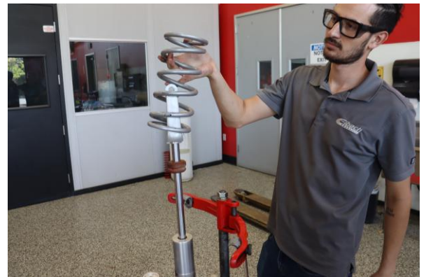
Install the Eibach Front Tender.
