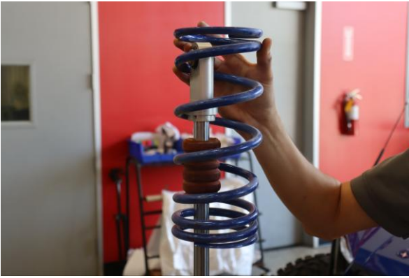
Remove the OE rear tender spring.
