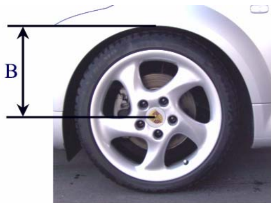
Measurement B Wheel hub center wheel arch
