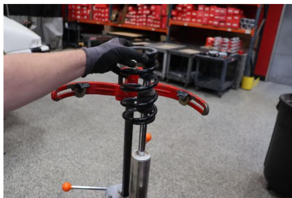
Step 10. Remove OE front secondary spring.
