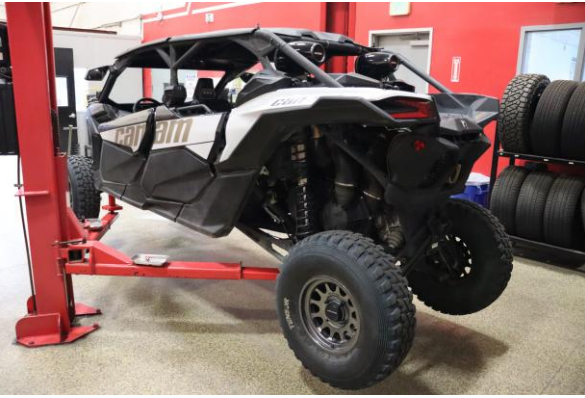
Step 1. Raise the rear of the vehicle and support it with the proper safety equipment.
