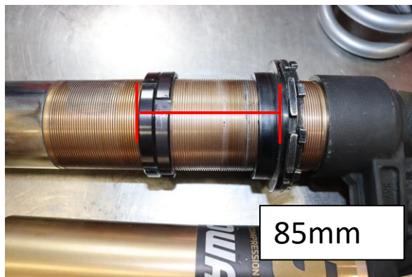
Step 12. Set crossover ring to 85mm (3 3/8in.) from bottom of spring seat to bottom of crossover ring.
