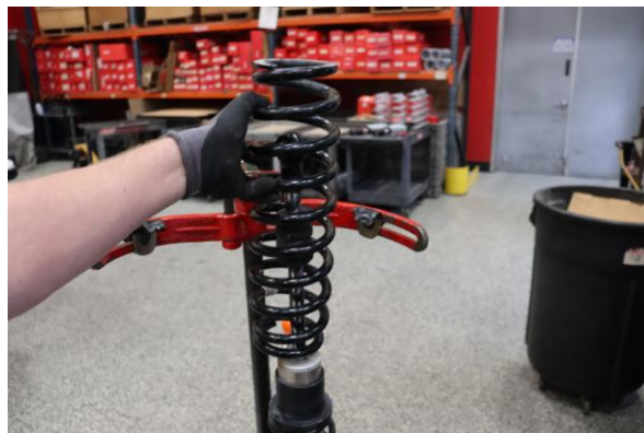
Step 8. Remove OE front main spring.
