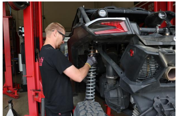
Step 18. Set shock assembly in vehicle by inserting top of assembly through opening in body panels and setting lower shock mount in trailing arm.
