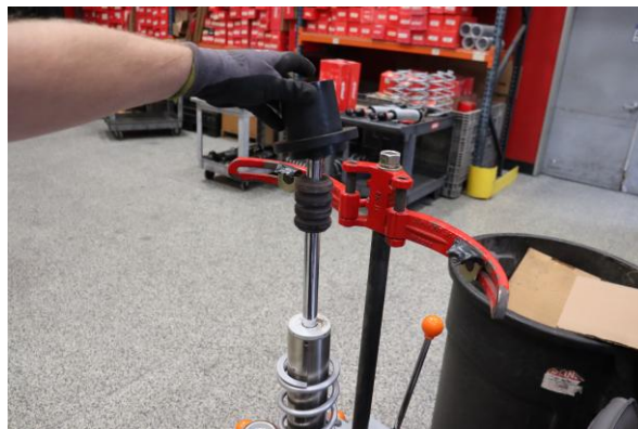
Step 14. Install EIBACH spring slider with larger face pointed away from secondary spring.
