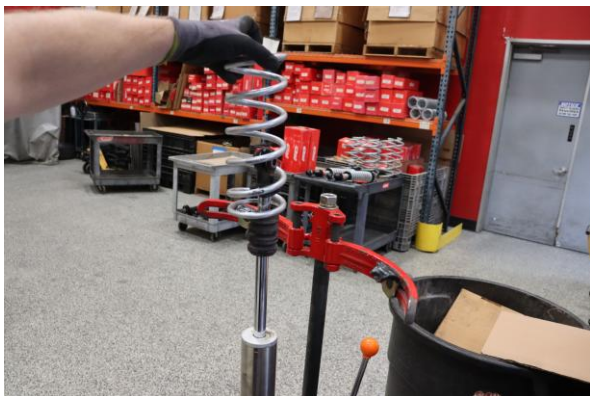
Step 13. Install Eibach front secondary spring.
