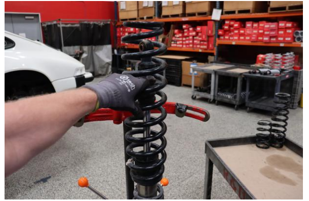
Step 8. Remove OE main spring.
