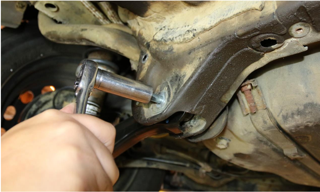
Remove the lower control arm bolt. (a)
