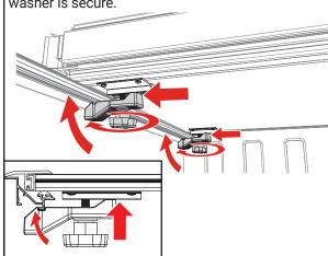
Unfold the cover (A) towards the tailgate. Then confirm each panel is centered side to side and front to back on the truck bed. If adjustments are needed, loosen the cover retainer clamps (E) and shift the cover (A) until positioned correctly. Retighten the cover retainer clamps once the desired fitment is reached. If adjustments to the slam latch are needed, see the directions on the next page.
