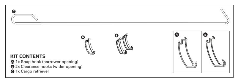
Lay out before Installation. Position the three hooks (A & B) in their approximate locations before snapping them into place. For best results, do this inside your truck bed or along the bed cap. It would be helpful to lay the cargo retriever where you want it and lay the according clips below in the instructions.
