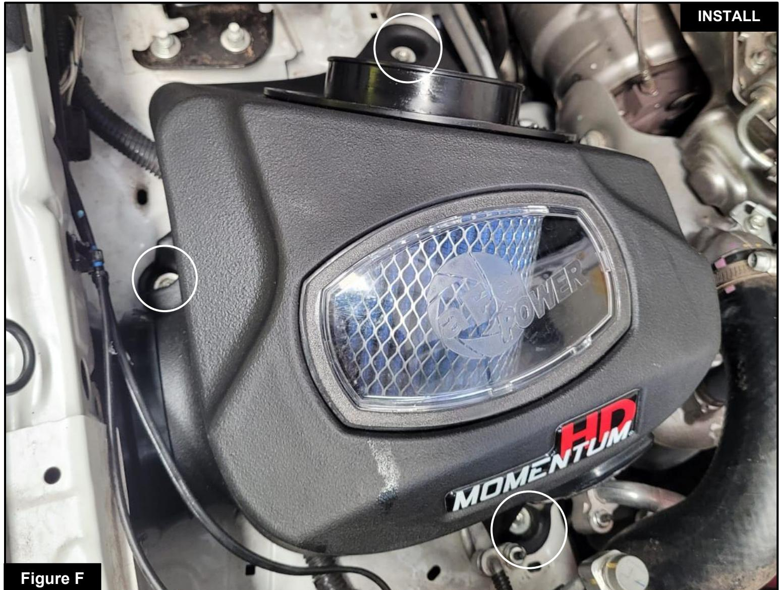
Step 11: Install the aFe POWER Housing into the truck and secure it with the 3 screws removed at step 4.
