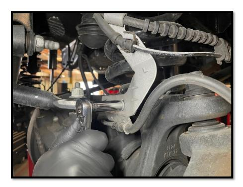
5. Using a **13mm** socket, remove the frame brake line bracket bolts.
