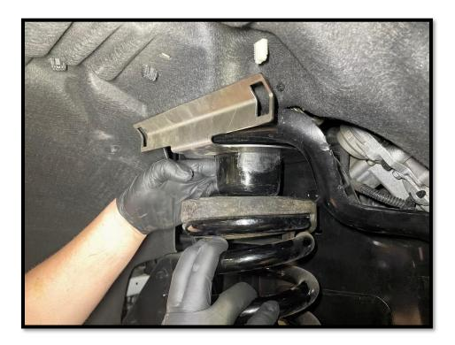
12. Verify that the lower spring pigtail is properly indexed with its axle seat as shown in the below photo.
