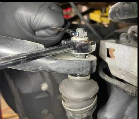
4. Using a **10mm** socket, remove the axle brake line bracket bolts.
