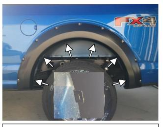
**STEP 6:** Place the Fender Flare onto the vehicle and fit into the correct position following the contours of the body. Use 6 of the U-style clips to secure the Fender Flare to the body. Make sure the barb in the clip securely attaches in the slot on the Fender Flare.
