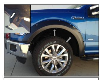
**STEP 3:** Place the Fender Flare onto the vehicle and fit into the correct position following the contours of the body. Use four (4) of the .6mm clips (two (2) per side) to secure the Fender Flare to the body. Make sure the dimple in the clip securely attaches in the slot on the Fender Flare.
