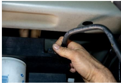
Figure 4: Removal of fuel feed line.
