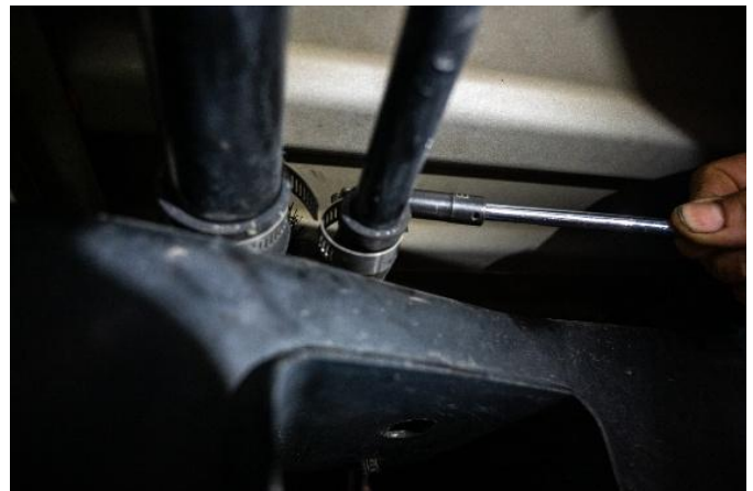
Figure 23: Fuel filler tube and fuel breather tube reinstalled.
