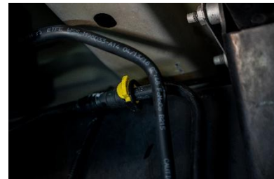
Figure 21: Reinstallation of fuel feed line.
