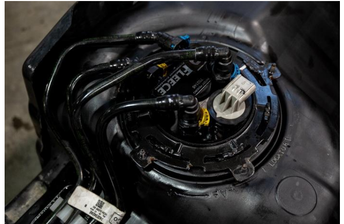
Figure 15: Fuel lines installed in same configuration as stock unit.
