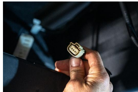
Figure 6: WIF sensor connector disconnected.
