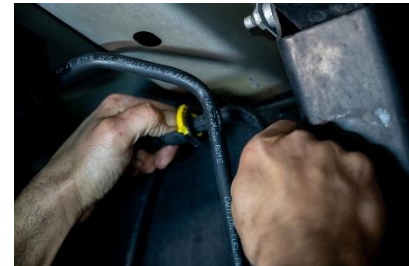
Figure 5: Removal of fuel return line.
