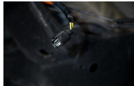
Figure 8: Stock lift pump electrical harness disconnected.
