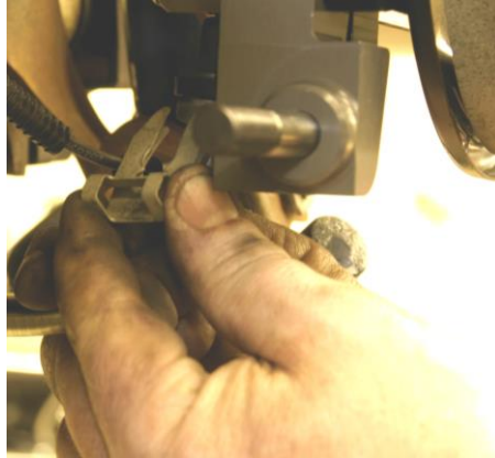
Figure 7: Cable retainer clip installation
