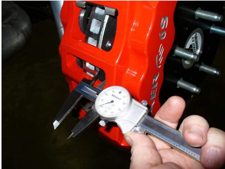
Figure 8: Measure gap from rotor to caliper body
