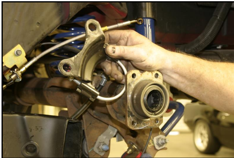
Figure 5: Remove brace and U-bolt
