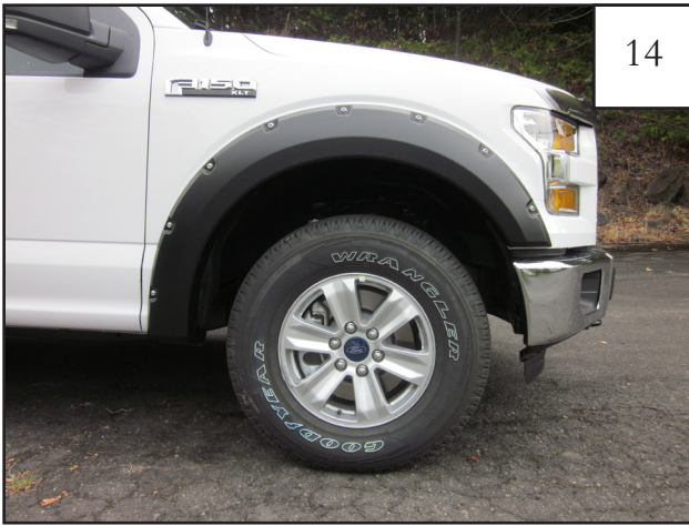
Completed front flare installation.
