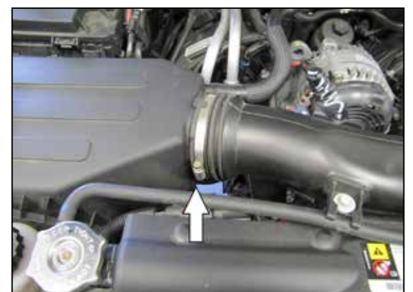
3. Loosen the hose clamp that secures the intake tube to the factory air filter housing.
