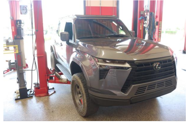
Step 25. Install both front wheels. Use 21mm to torque lug nuts to factory specification. (97 ft-lb) when vehicle is on ground.
