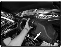
**4.** Un-clip the upper half of the air box attached to bottom of air box. Remove stock assembly out of vehicle.
