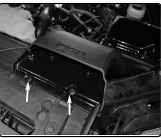
**13.** Re-use the two plastic retaining rivets from figure 2 to secure the Injen lower air box scoop to the radiator support
