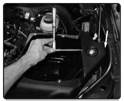
**12.** Use the OE air box bolt to secure the lower Injen air box to the chassis
