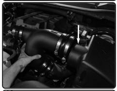
**18.** Install the Injen intake tubeto the factory intake tubes and then connect the Injen intake tube the the Injen intake air box. make your final adjustment and then secure all the clamps
