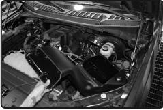
11. Lower the Injen lower air box into the engine bay. Make sure you line up the stand offs on the bottom side of the Injen lower air box to the grommets on the chassis.
