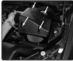
15. Place the plenum onto the top of the Injen lower air box. Use 4-M6X20 bolts to secure the plenum to the Injen lower air box
