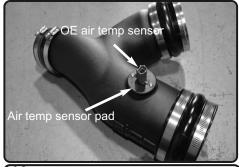
**16.** Use the supplied M4 bolts to secure the Molded air temp sensor pad onto the Injen intake pipe and then push the AIT sensor into the sensor pad and twist to secure the AIT sensor to the sensor pad
