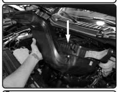
7. Now lift up and remove the bottom half of air box out of vehicle.
