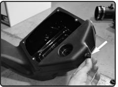
**9.** Remove the grommet and spacer from the OE lower air box and re-install it in the Injen lower air box.
