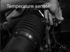
7. Disconnect the temperature sensor harness.
