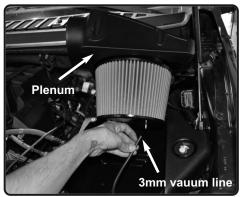
14. Place the filter onto the Injen plenum and connect the 3mm vacuum line from the Filter Minder to the barbed fitting on top of the filter
