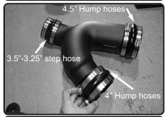
**16.** Place the supplied hoses illustrated in the photo. The # 72 clamp will be used on the 4.0" and 4.5" hump hoses and #64 and #56 clamps will be used for the 3.5"-3.25" step hose.
