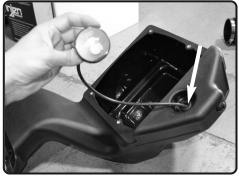
**10.** Install the supplied grommet into the Injen lower air box and then push the 3mm vacuum line and Filter Minder through the grommet.
