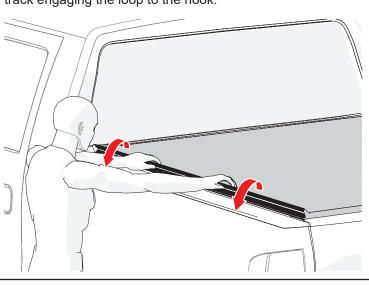
the hook and loop engaged, use the palms of your hand to firmly push the loop strip into the hook track. Do this to both driver and passenger sides. You are ready to drive with the cover (C) in the closed position.
