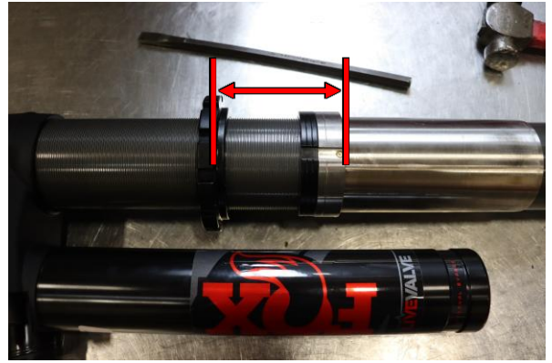
Step 14. Set crossover ring to 110mm (4 5/16in.) from bottom of spring seat to bottom of crossover ring.
