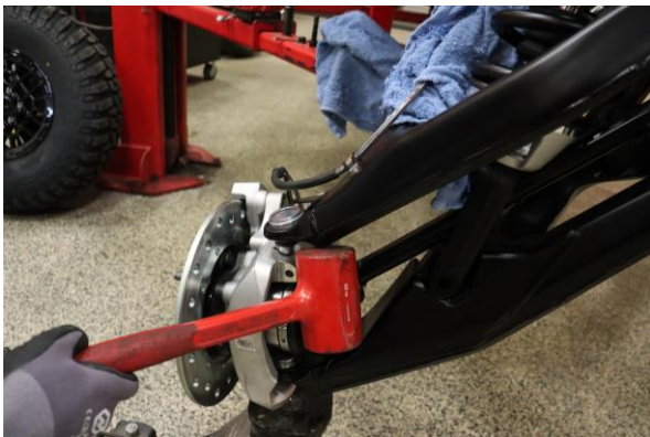
Step 5. Carefully release the upper control arm from the top of the spindle.
