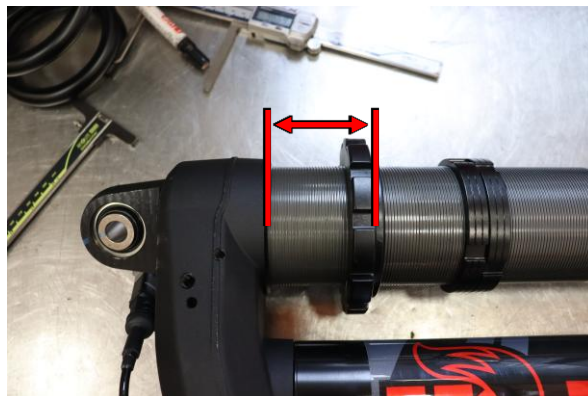
Step 14. Set pre-load of spring seat to 80mm (3 3/16in.) from bottom of seat to bottom of reservoir bridge.
