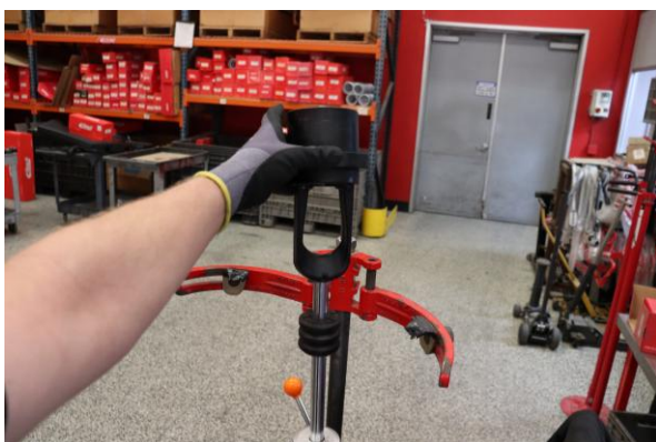
Step 17. Install the OE spring slider with the larger end facing away from the secondary spring.
