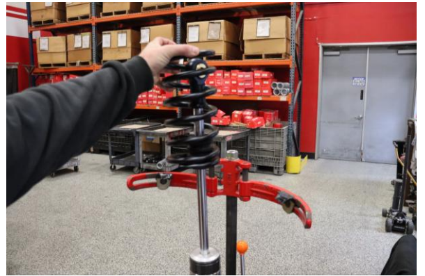
Step 10. Remove the OE rear secondary spring.
