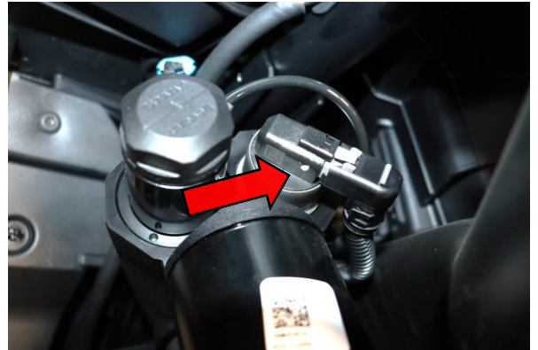
Step 21. Reconnect both compression and rebound electrical connectors.
