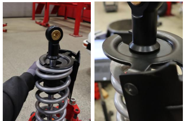
Step 18. Compress the spring assembly and install the lower spring perch. Decompress the spring assembly making sure that the lower spring perch seats fully against the lower shock mount.
