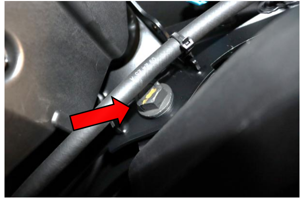
Step 20. Use two 21mm to install the upper shock mount bolt. Tighten to manufacturer specification.
