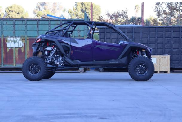
Step 22. Lower the vehicle and carefully test drive while listening for any abnormal noises. Measure from the ground to the center of the skid plate between the rear mount of the front lower control arms. The recommended preload measurement in Step 13 will get the vehicle close to the recommended ride height but each vehicle may vary some. We recommend setting the ride height at 407mm (16in.) measuring from the ground to the center of the front skid plate/ ground clearance. Note: Measurements were taken from a vehicle with 32in. tires. If your vehicle has a different size tire, the ride height will need to be adjusted. Due to the sensitivity of weight of these vehicles, weight distribution may change ride heights, additional pre-load may need to be added to compensate.
