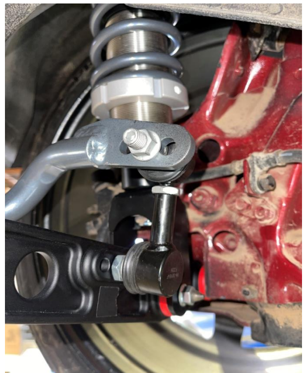
(T) Install with aftermarket aluminum LCA
