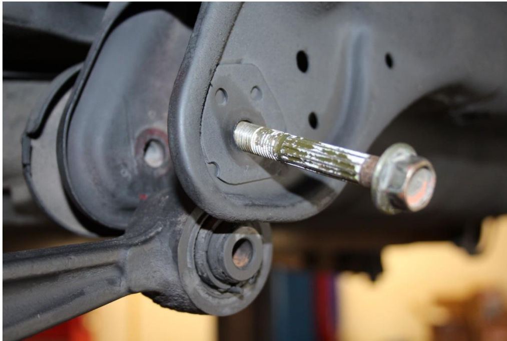
(A) Remove the Lower Control Arm bolt
