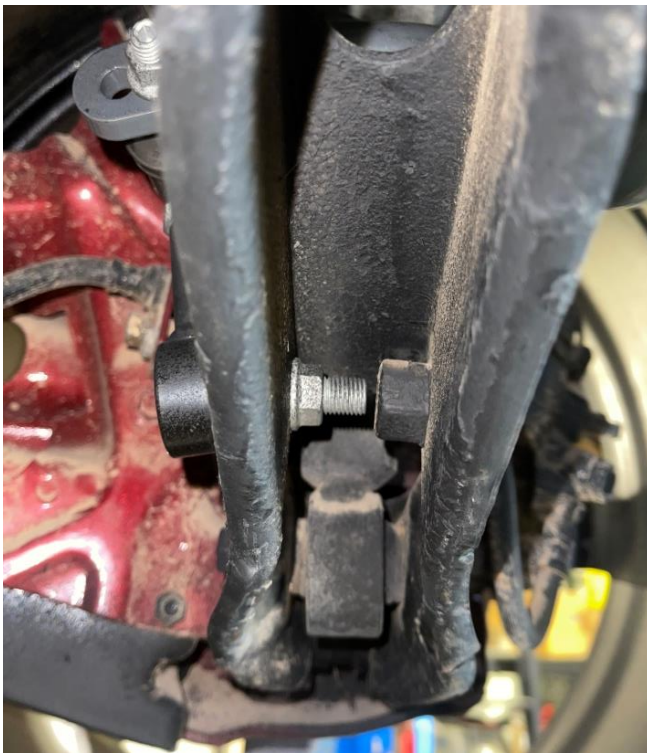
(S) Install with stamped steel LCA
