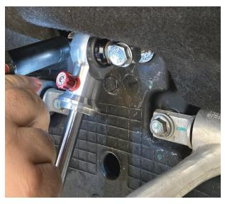
Fig. 7: Tighten the upper shock bolts.
