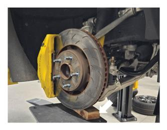
Fig. 1: Support the suspension.
