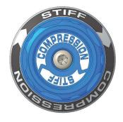
Low-Speed Compression (LSC) for general platform control from driver inputs and gradual road inputs. Too little LSC can cause a loose/soft feeling car. Too much LSC can increase harshness and reduce grip (especially in slick conditions). Adjust by turning the knob.
