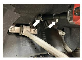
Fig. 3: Remove the upper shock bolts.
