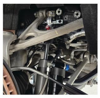
Fig. 14: Install the shock; rebound adjuster facing away from frame, hose facing outboard.
