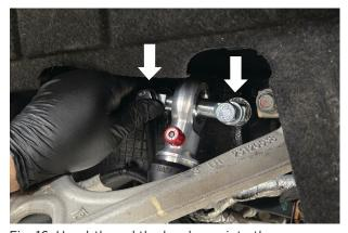
Fig. 16: Hand-thread the hardware into the upper shock mount.
