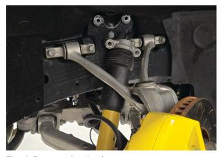
Fig. 4: Remove the shock.
