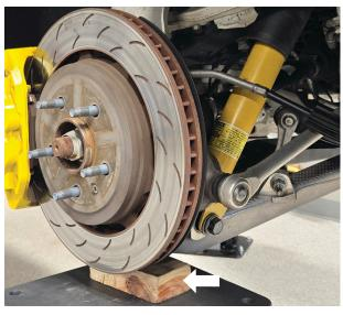
Fig. 11: Support the suspension.
