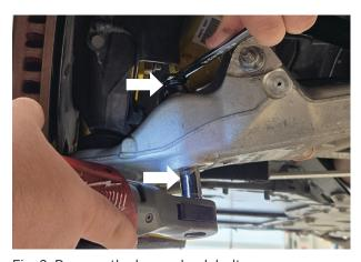
Fig. 2: Remove the lower shock bolts.
