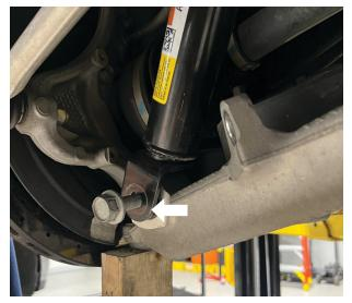
Fig. 12: Remove stock lower shock bolt.
