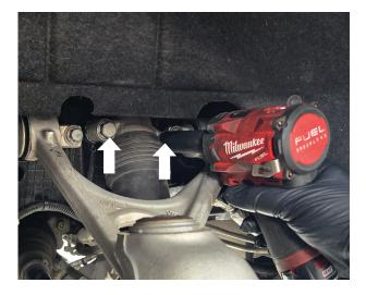
Fig. 13: Remove the stock upper shock bolts
