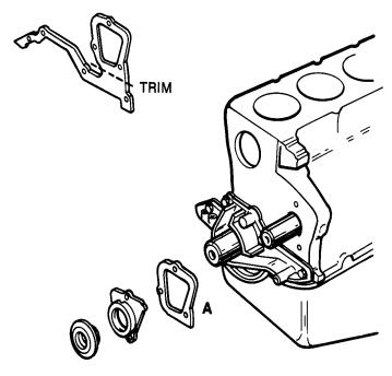
Trim seal holder gasket to fit, if required, and cement in place on engine casting surface using adhesive. "A"
