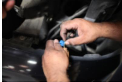
Splice the two twisted black wires from the Anzo headlight to the black wire from the harness
