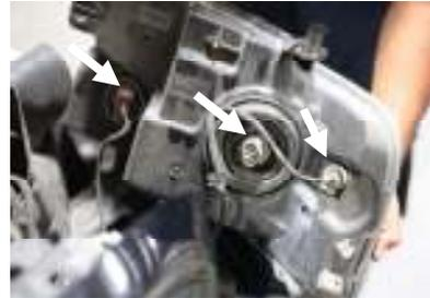
Connect the headlight, signal, and side marker harness into its power source sockets
