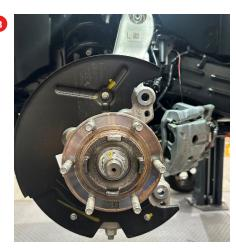
2 HOLD UP 6-POT CALIPER TO BACKING PLATE. USE A PAIN PEN MARK CLEARANCE CUT LINE.
