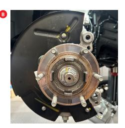
4 AFTER TEST FITTING THE BACKING PLATE, CHECK TO SEE IF THE O.E. HUB CASTING IS TOUCHING THE CALIPER. IF IT IS, MARK CONTACT POINTS AND REMOVE EXCESS CASTING.
