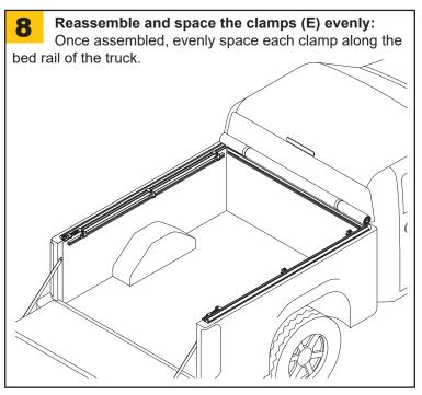
Positioning of clamps (E) at the cab: The front clamps will use the inner groove to properly position the side rails at the front of the truck bed.
