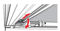
With the tailgate open, pull cord downward on one side to disengage both slam latches from both sides.
