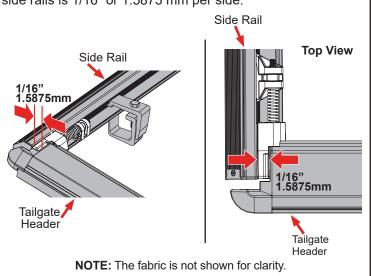
Positioning of clamps (E): The clamps positioned near the tailgate will use the outer groove.
