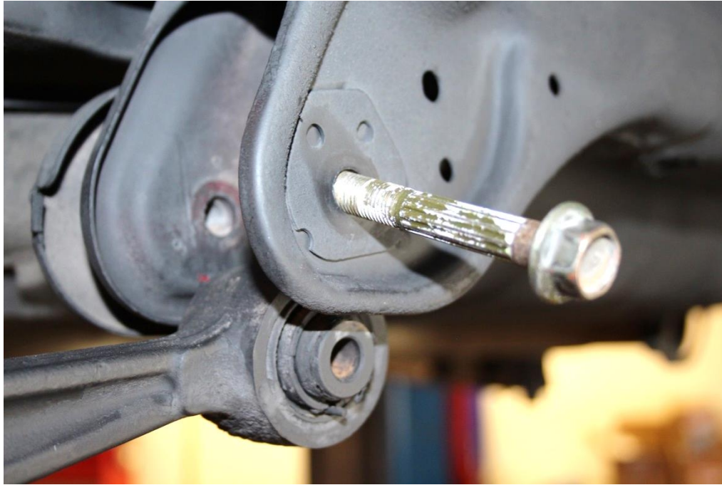
(A) Remove the Lower Control Arm bolt
