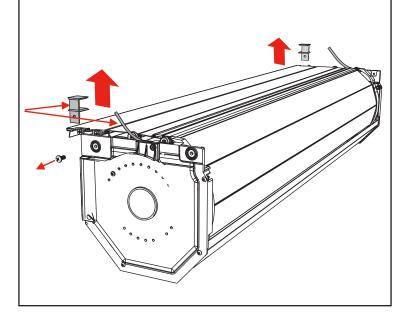
Install the rails to the canister: Pull the cover out of the canister (D) 6 to 8 inches, holding it from rolling
