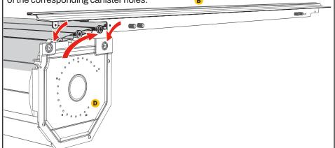
Fasten the rails to the canister: With the rails in place and the cover slid into the rail channel, attach the rails with the four 10-32 x 7/16" canister mounting screws (E).
