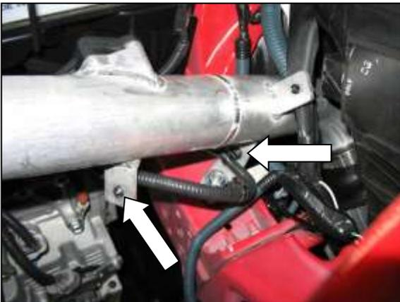
n. Route the MAF sensor connector wire harness under the intake pipe as shown. Secure the harness in two places using the remaining two push-mount zip ties.
