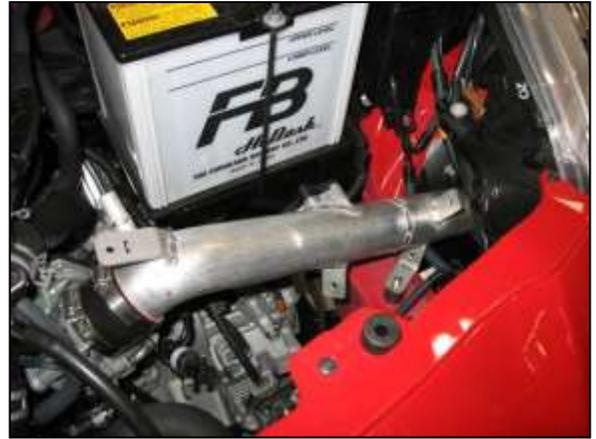
e. Install the AEM® intake pipe into the engine bay. Align the mounting bracket onto the rubber mount installed in step 3b. Insert the other end of the intake pipe into the coupler installed on the throttle body.
