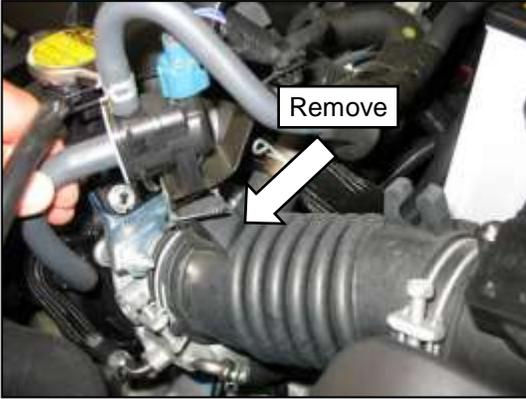
c. Pull the EVAP VSV mounting clip free from the intake tube. Remove the Phillips head screw that secures the mounting bracket to the EVAP VSV.
