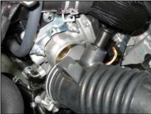
e. Loosen the hose clamp and pull the intake tube clear of the throttle body.
