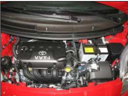
a. Factory airbox system installed.
