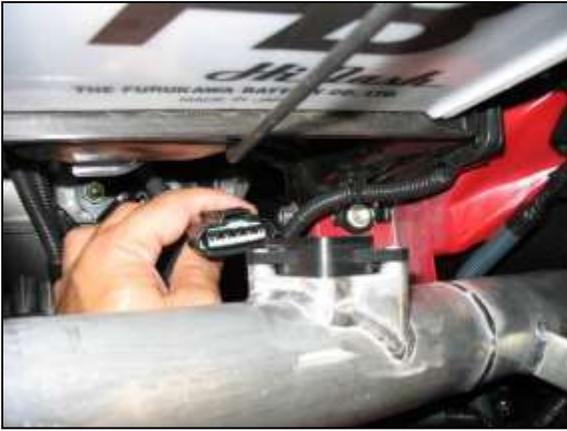
l. Plug in the MAF sensor connector to the MAF sensor.
