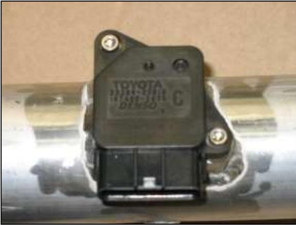
d. Install the MAF sensor into the AEM® intake pipe. Secure with the two provided 8-32 socket bolts. Use care during the installation to avoid damaging the o-ring.
