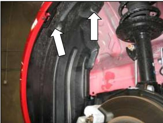
j. Remove the two plastic rivets by popping up the center with a small screwdriver. Pull the fender liner back to expose the inner bumper area.
