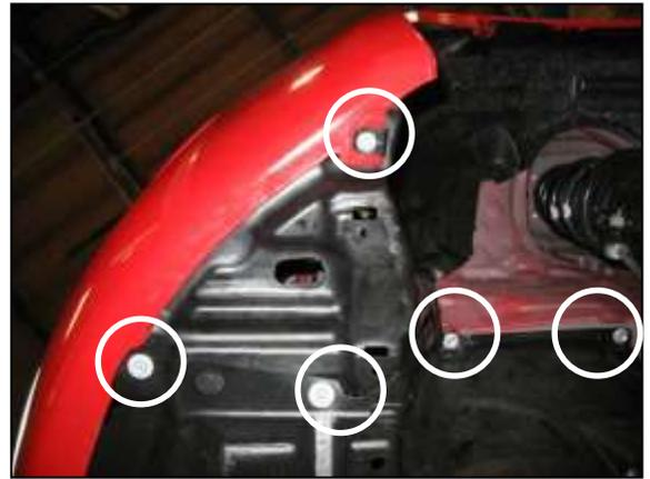
i. Raise the front of the vehicle with a jack. Refer to your owner's manual for proper jack and jack stand placement to properly support vehicle. Support your vehicle using properly rated jack stands before wheel removal or while working under the vehicle. **NEVER WORK UNDER A VEHICLE WITHOUT USING JACK STANDS.** Remove the driver side wheel. Remove the five screws securing the lower splash guards.
