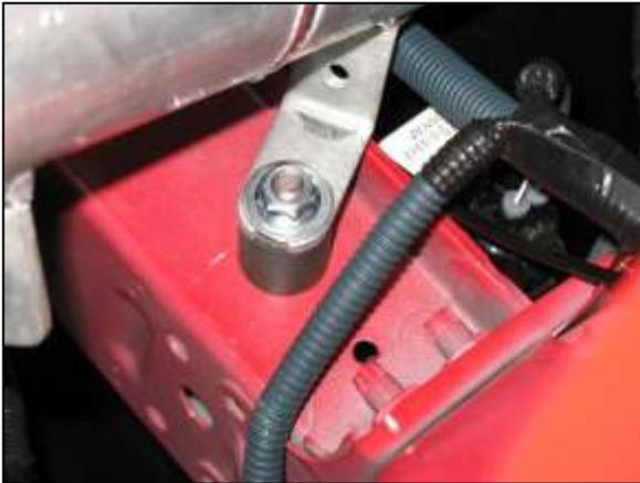
f. Loosely secure the pipe's mounting bracket to the rubber mount with the supplied M8 washer and nut.
