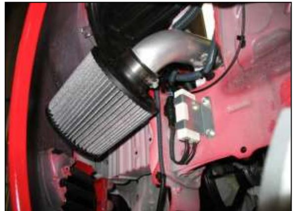
k. Install the AEM<sup>®</sup> air filter onto the end of the intake pipe. Slide it on until the shoulder inside the air filter is flush with the end of the pipe. Secure with the supplied 2.15-3.00" hose clamp.
