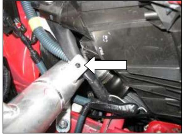
m. If the wire harness behind the headlight rubs the intake pipe, secure it to the mounting tab with one of the supplied push-mount zip ties. Ensure the wire harness is NOT in tension. Depending on the length of the wiring harness, this step may not be necessary.
