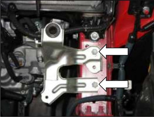
i. Remove the two bolts securing the airbox mounting bracket. Release the wire harness clip from the underside of the airbox mounting bracket. Remove the airbox mounting bracket from the engine bay.
