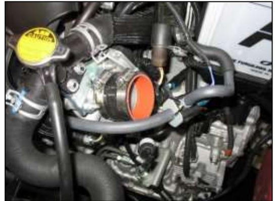
c. Install the silicone coupler onto the throttle body. Loosely install the two 2.25" hose clamps.
