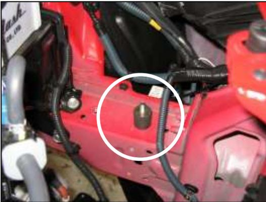
b. Install the M8 rubber mount into the forward-most airbox bracket mounting hole.
