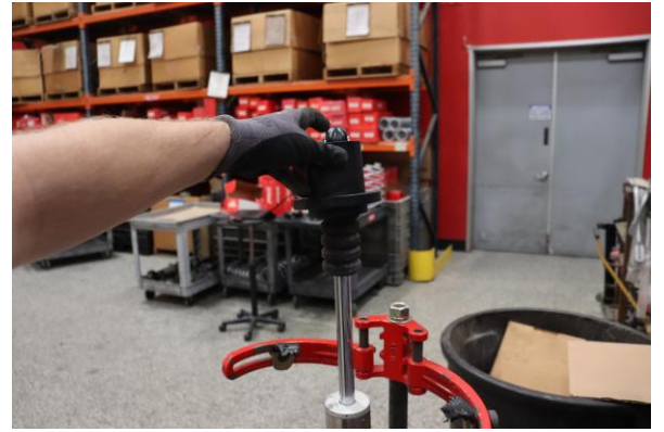
Step 14. Install EIBACH spring slider with larger face pointed away from secondary spring.
