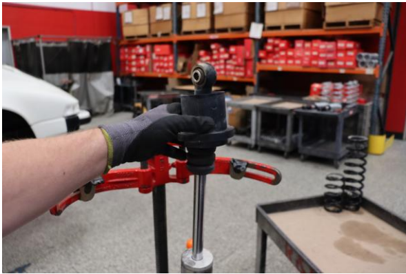
Step 9. Remove OE spring slider.
