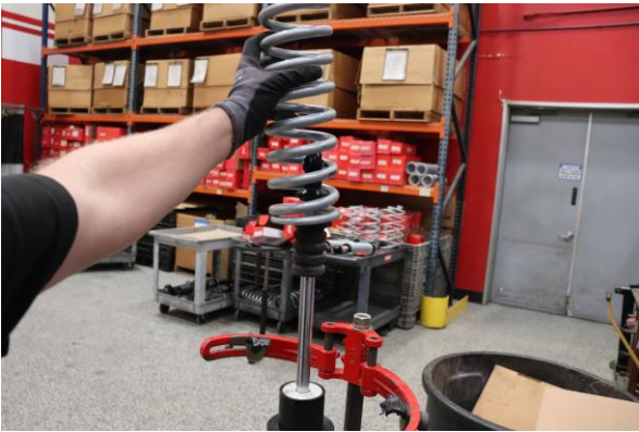
Step 15. Install Eibach rear main spring.
