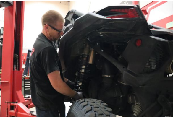
Step 5. Lift and remove the shock assembly from the bottom shock mount first then lower shock from car.
