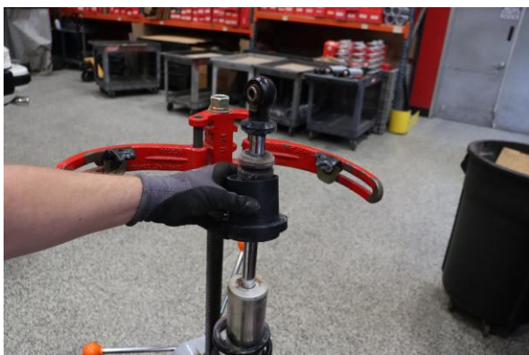
Step 9. Remove OE slider.
