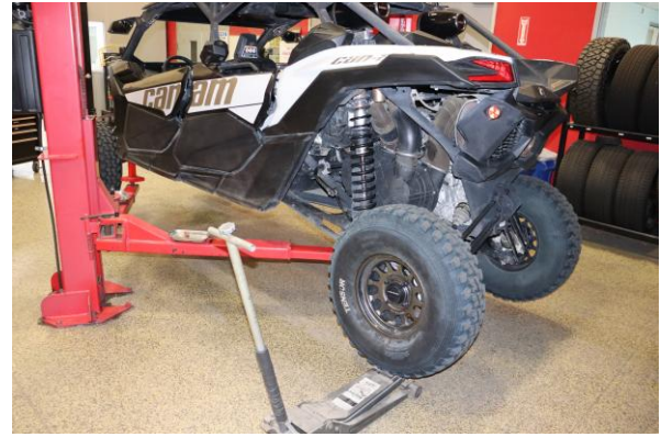
Step 2. Support weight of wheel and tire with floor jack.
