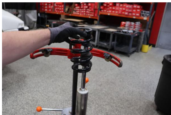
Step 10. Remove OE front secondary spring.
