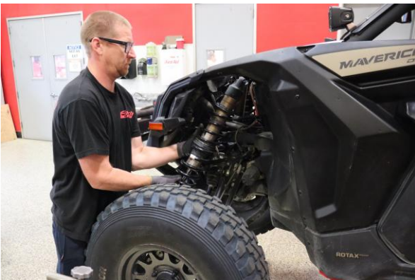
Step 5. Lift shock to clear lower shock mount and lower shock to remove from car.
