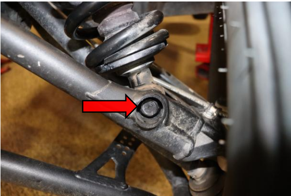
Step 3. Remove 18mm lower shock nut and bolt. Need 2 18mm sockets
