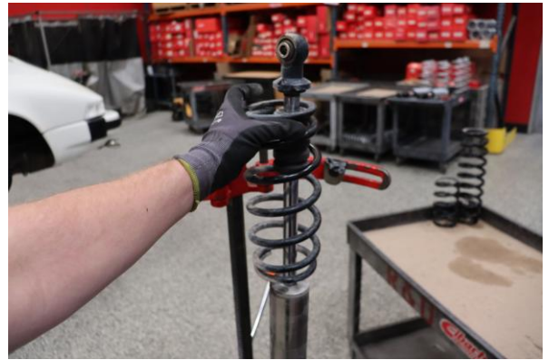
Step 10. Remove OE secondary spring.
