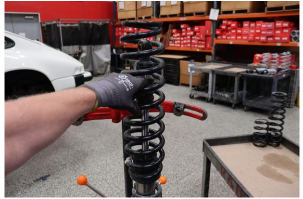
Step 8. Remove OE main spring.
