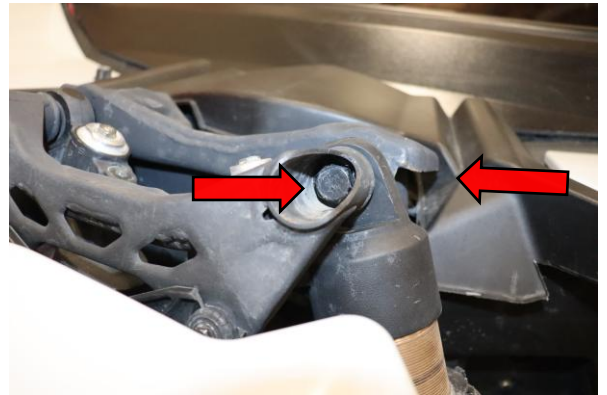
Step 4. Remove 18mm upper shock bolt and nut from both left and right front. Need socket and wrench.
